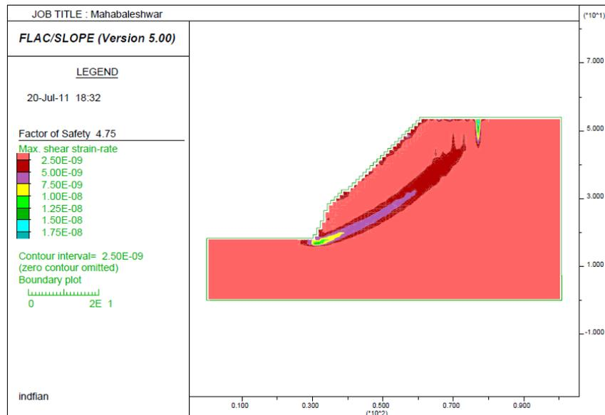
Figure 3: An analyzed slope showing shear strain and development of tension crack.
