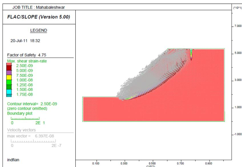
**Figure 4:** An analyzed slope showing velocity vectors of the grains of rock mass.
