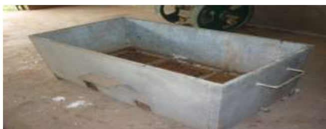
Fig. 1: Direct Convictional Steam Treatment Chamber for Whip Smut Control.
