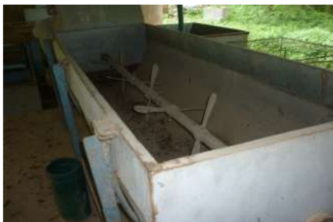
Fig. 7: Air Cool Crystallizer System
