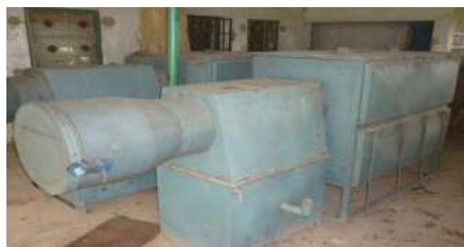
Fig. 2: Indirect Forced Air Steam Treatment Chamber for whip Smut Disease Control in Sugar Cane
