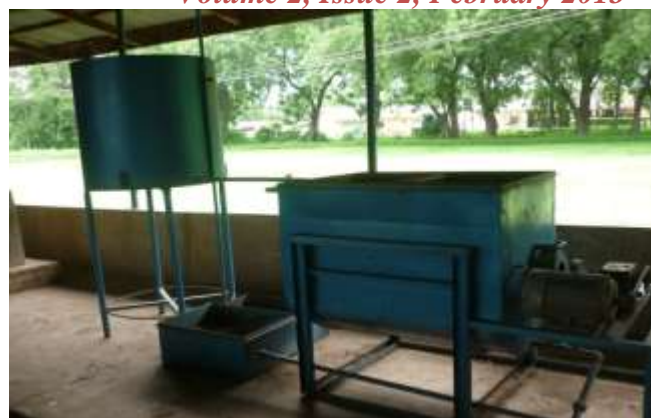
Fig. 8: Combined Air/Water Cool Crystallizer System
