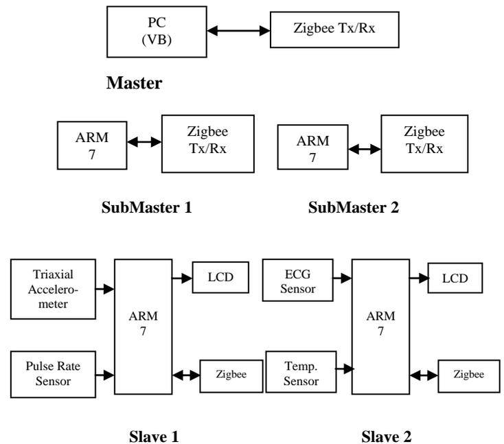
Figure 1. Block Diagram of Wireless Patient Monitoring
