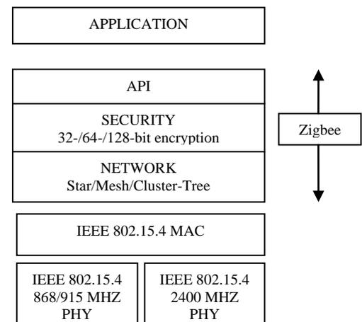
**Figure2. Architecture of Zigbee/IEEE 802.14.5**
