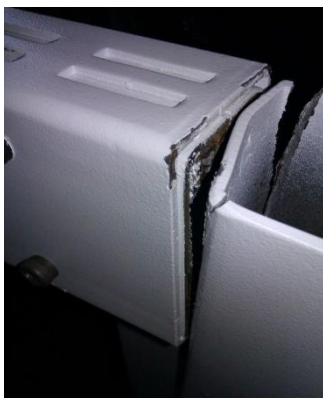
Fig.2 Failure of upright & base
