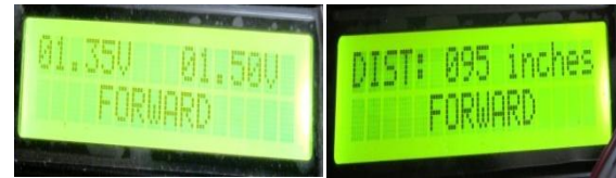
Figure 12: ALCD display of the controller and robot when transmitter is in manual mode and when tilted ahead.
