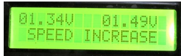
Figure 13: ALCD display of the transmitter commanding the robot to increase its speed.
