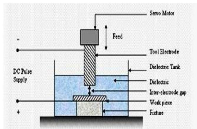
Figure 1(a) Servo system of EDM
