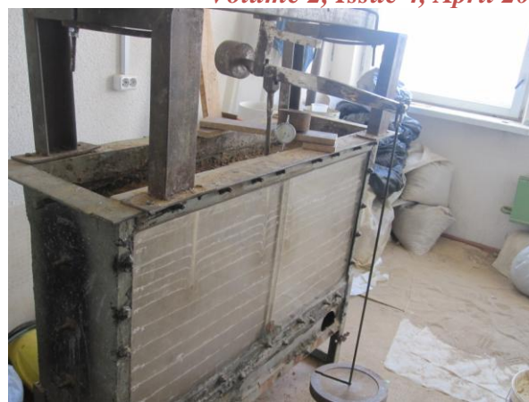
Figure 1. Tank set up and load application on the Soil
