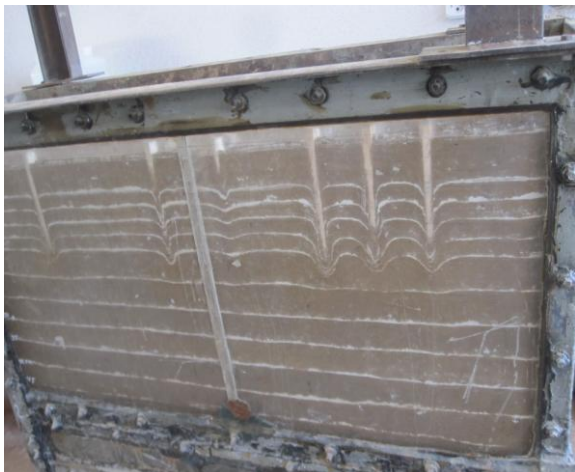
Figure 8. Testing Tank showing eaves, depression and settlement of piles
