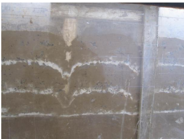
Figure 9. Failure bulb and Deformation Zones under load
