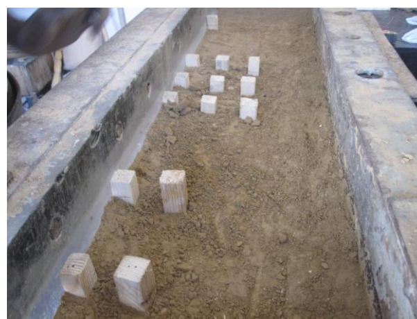
Figure 2. Pile driven into Clay Soil in the Tank
