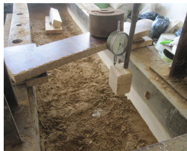
Figure 3. Settlement measurement on Dial gauge
