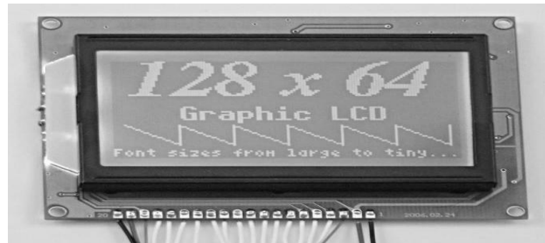
Fig2.4: 128x64 Graphic LCD
