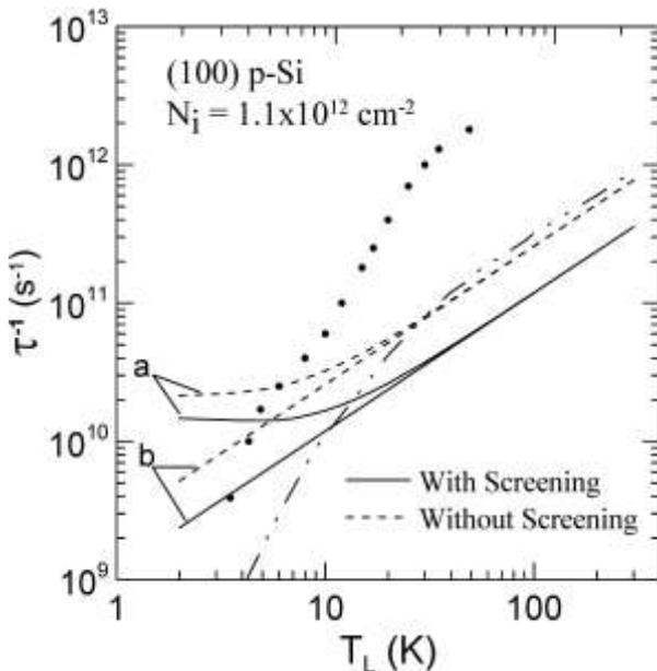
**Fig.2 :** Lattice temperature dependence of intravalley acoustic phonon scattering rate of free electrons with Fermi energy in (100) Si inversion layer. Symbols are from Experiment [11], dash-dot curve is from the theory of Shinba and Nakamura [12]. Letters a and b indicate respectively the contribution from the full phonon spectrum and its equipartition approximation.
