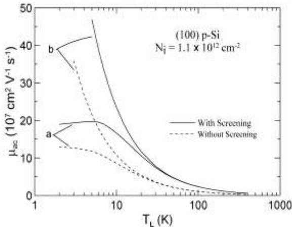
**Fig.1 :** Lattice temperature dependence of intravalley acoustic phonon limited zero-field electron mobility in (100) Si inversion layer. Letters a and b indicate respectively the contribution from the full phonon spectrum and its equipartition approximation.
