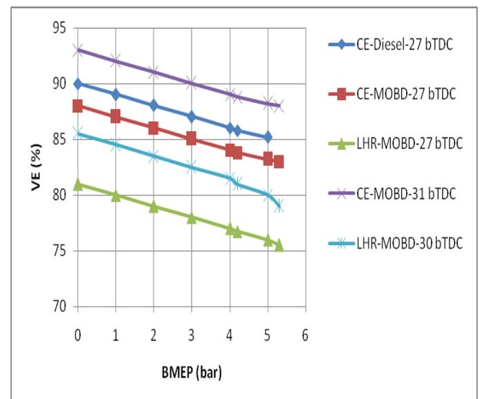
Fig.6 Variation of volumetric efficiency (VE) with BMEP in CE and LHR engine at recommend injection timing and optimized injection timings with biodiesel (MOBD) operation at an injection pressure of 190 bar.
