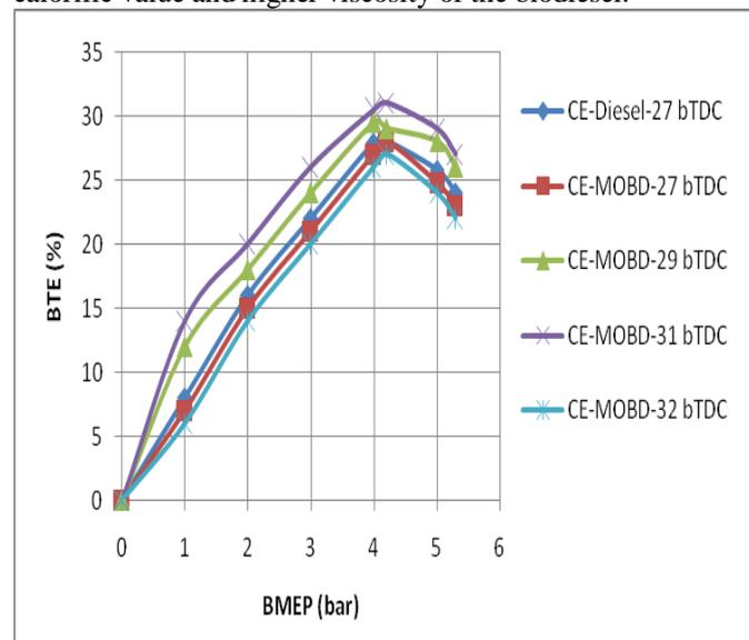
Fig.2 Variation of brake thermal efficiency (BTE) with brake mean effective pressure (BMEP) in conventional engine (CE) at different injection timings with Mohr oil based biodiesel (MOBD) oil operation at an injection pressure of 190 bar.
