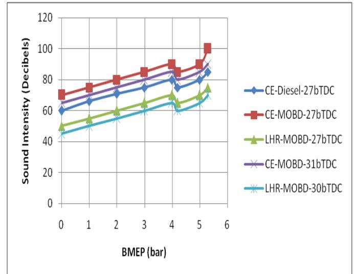
Fig.8 Variation of sound intensity with BMEP in CE and LHR engine at recommend injection timing and optimized injection timings with biodiesel (MOBD) operation.
