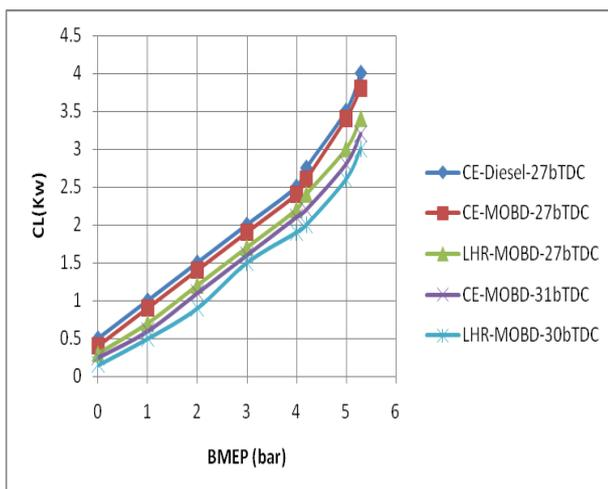
Fig.7 Variation of coolant load (CL) with BMEP in both versions of the engine at recommended and optimized injection timings with MOBD operation at an injection pressure of 190 bar
