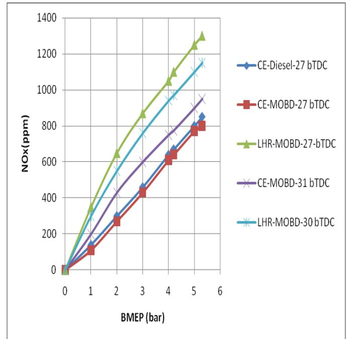
Fig.9 Variation of NO<sub>x</sub> levels with BMEP in CE and LHR engine at recommend injection timing and optimized injection timings with biodiesel (MOBD) operation at an injection pressure of 190 bar.
