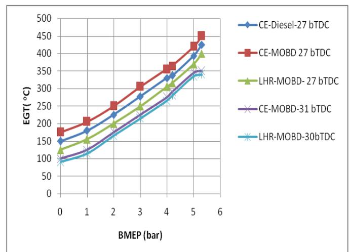
Fig.5 Variation of exhaust gas temperature (EGT) with BMEP in CE and LHR engine at recommend injection timing and optimized injection timings with biodiesel (MOBD) operation.
