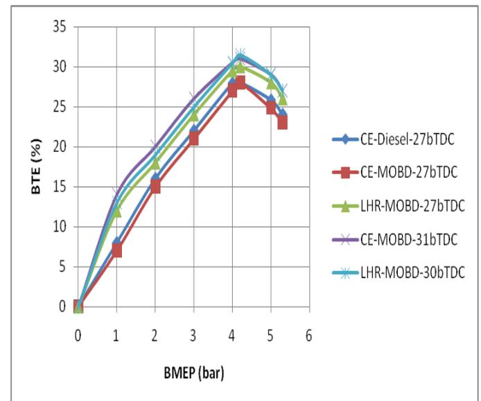
Fig.4 Variation of BTE with BMEP in different versions of the engine at the recommended injection timing and optimum injection timing at an injection pressure of 190 bar.
