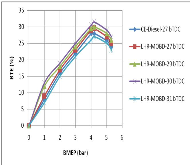
Fig.3 Variation of BTE with BMEP in LHR engine at different injection timings with biodiesel (MOBD) operation.
