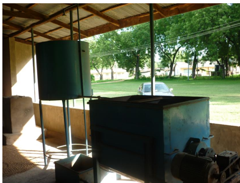
Plate 3: Combined water and Air cool crystalizer
