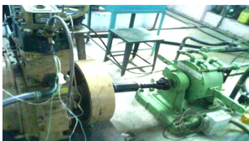
Fig - 1 - Engine coupled with eddy current dynamometer
