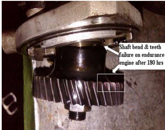
Fig1 Teeth Failure of Gear
