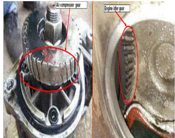
Fig.5 air compressor teeth failure
