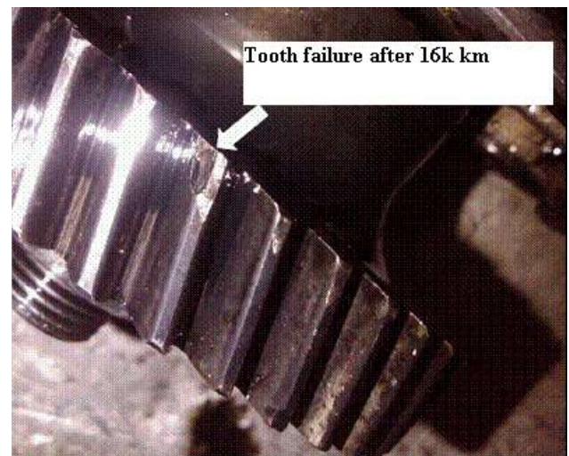
Fig.3 teeth failure camshaft gear after 16k km running.
