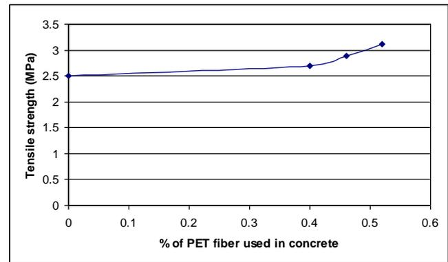
Fig. 5 Variation of tensile strength with different percentage of PET fibres.
