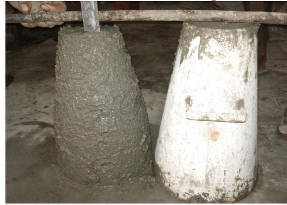
Fig.2 Slump Test
