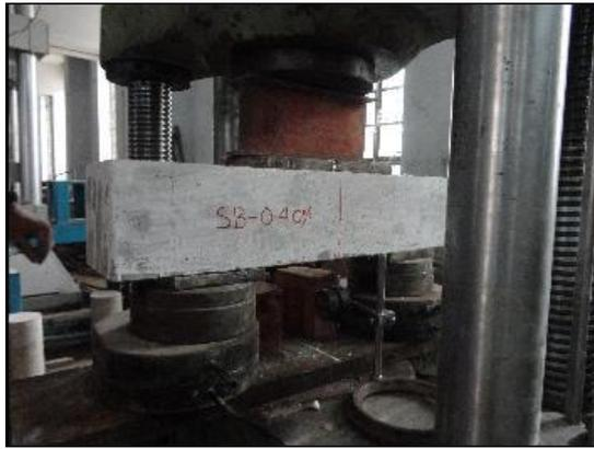
Fig. 4 Shear capacity test of beam.
