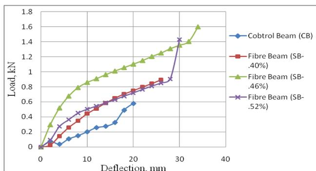
Fig. 8 Load versus deflection curves from direct shear test.
