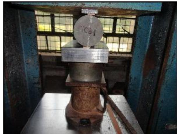
Fig.3 Splitting tensile strength test
