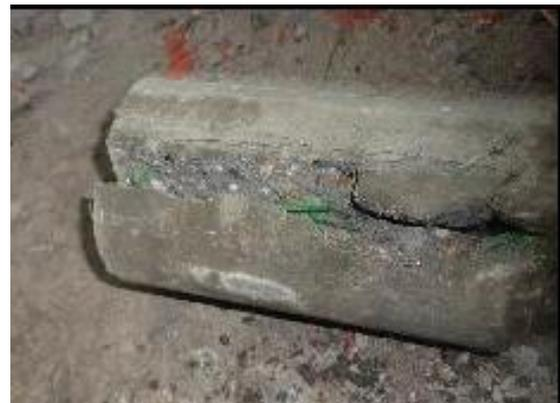
Fig. 6 Failure Pattern of cylinder specimen.
