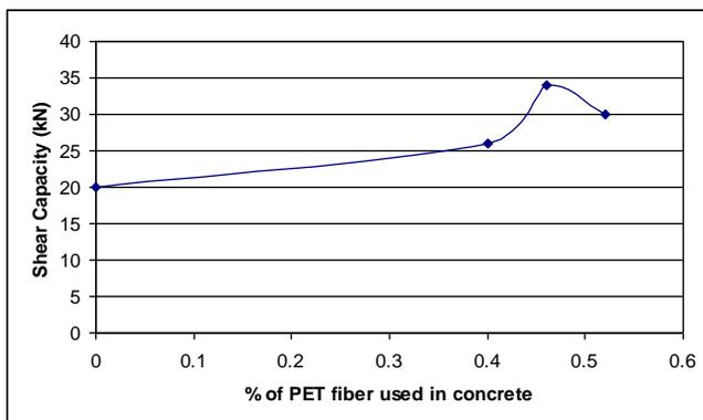
Fig. 7 Variation of shear capacity with different percentage of PET fibres.
