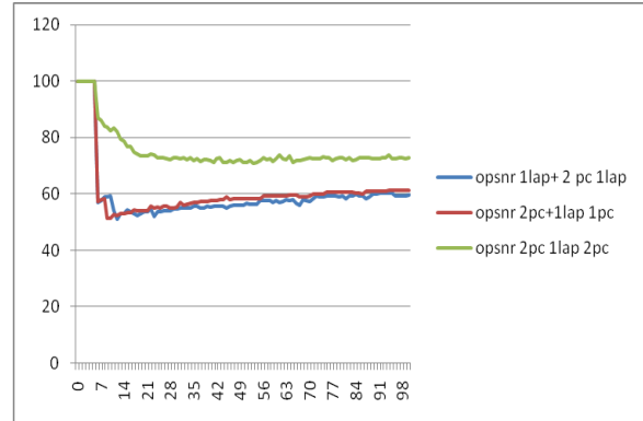
Fig 6: PSNR of real time video streaming for multiple accesses, compared with existing video played on the same machine
