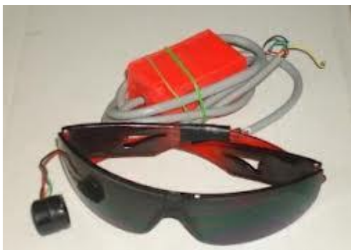
Fig.2: Module for Eye Blinks Detection.
