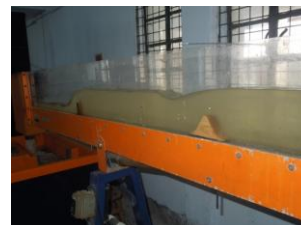
Fig. 3 Pictorial view of laboratory tilting flume
