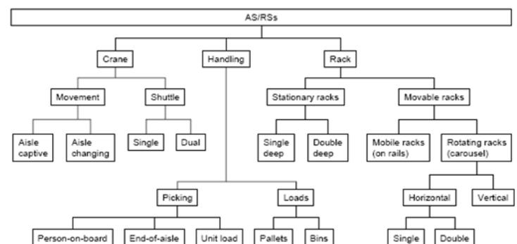
Figure 1:- different types for automated storage and retrieval system
