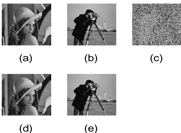
Fig.6) (a) is original image, (b) is original watermark image, (c) is the watermark image after chaos with optimized GA encryption, (d) is the watermark embedded image and (e) is the watermark image after extraction and decryption process.
