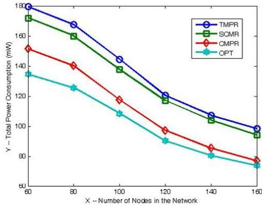
Fig. 2. energy utilization vs. number of nodes in the system.
