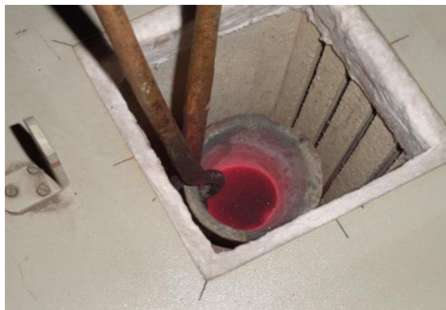
Fig 2.3 Preheated Mixer of SiC and Graphite Powder
