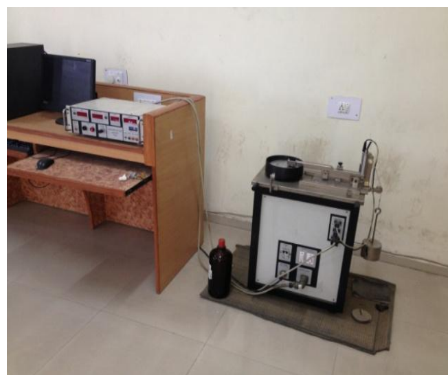
Fig 3.1 Pin on Disc Machine for Wear Test Al/SiC/Gr MMHC
