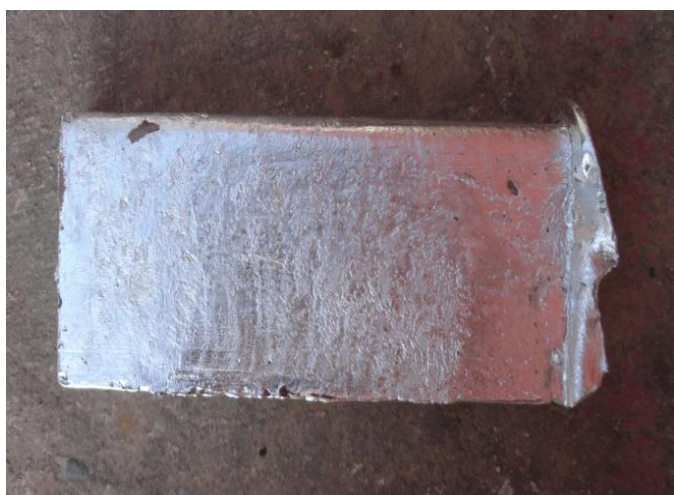
Fig 2.4 Prepared Al/SiC/Gr MMHC
