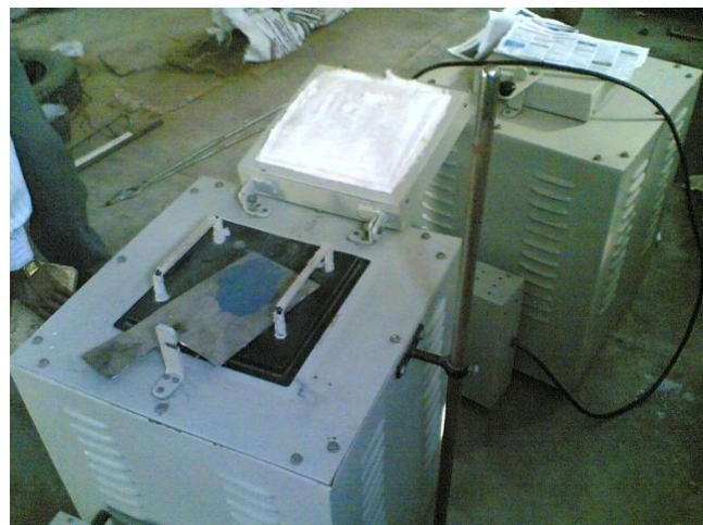
Fig 2.1 Muffle Furnace used for Fabrication of Hybrid Composite
