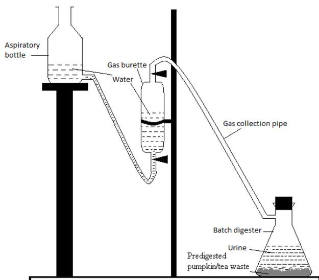
**Fig. 1.** Schematic diagram of digester set-up for pumpkin or tea waste [26]
