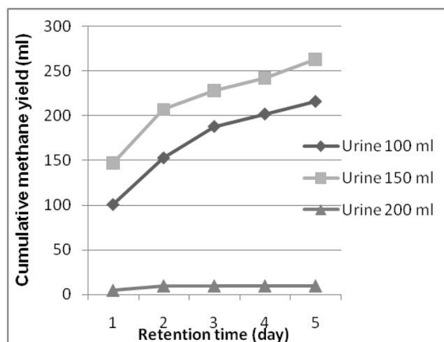
**Fig. 3.** Cumulative  $\text{CH}_4$  yield (ml) against retention time (day) at different levels of urine from pumpkin waste
