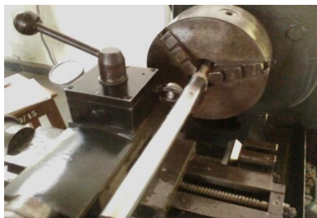
Figure 1: Experimental set-up for burnishing process.
