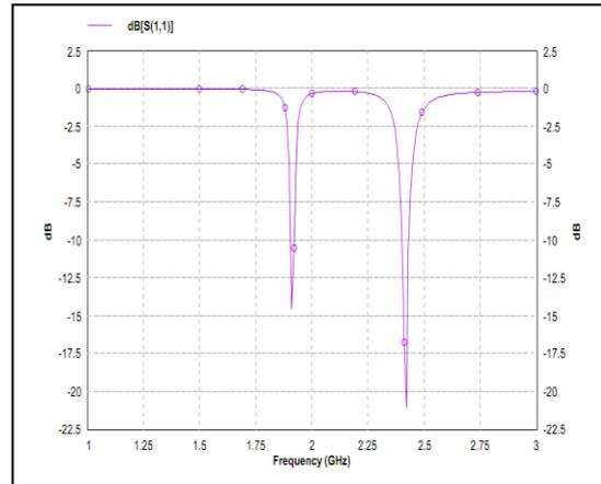
**Fig.3.** Return loss vs. frequency graph of Circular cut shape of rectangular microstrip patch antenna
