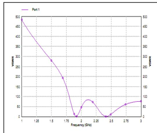
**Fig.4.** VSWR vs. frequency graph of Circular cut shape of rectangular microstrip patch antenna
