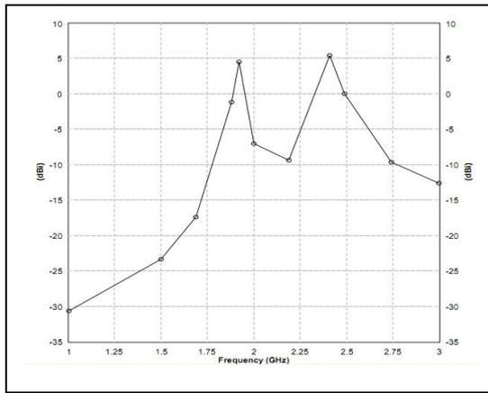
**Fig.5.** VSWR vs. frequency graph of Circular cut shape of rectangular microstrip patch antenna
