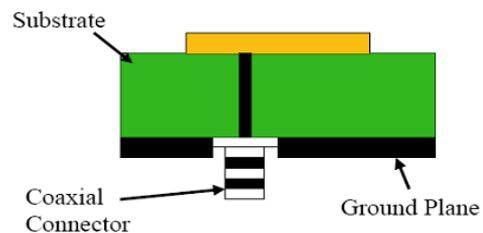
Fig.1 Coaxial probe feed via. SMA connector
