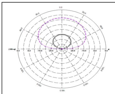
**Fig.7.** 2D Radiation pattern of Circular cut shape of rectangular microstrip patch antenna at 2.42 GHz.
