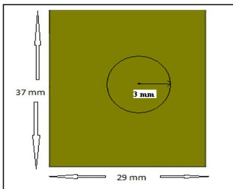
**Fig.2.** Circular cut shape of RMPA
