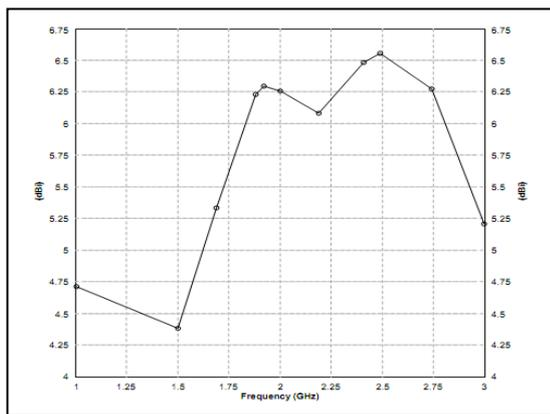
**Fig.6.** Directivity vs. frequency graph of Circular cut shape of rectangular microstrip patch antenna
