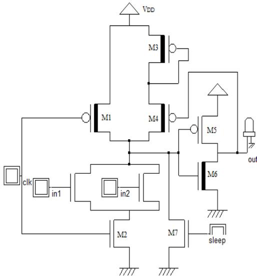
Fig .4. Sleep switch based domino circuit
