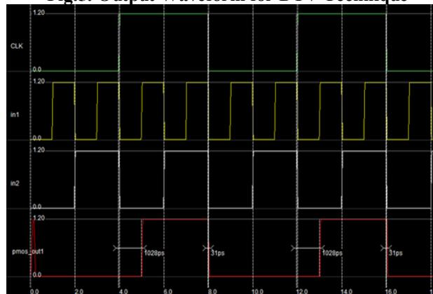
Fig.6. Output Waveform for STDTV Technique
