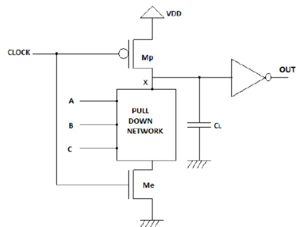
**Fig.1. Basic domino logic circuit**
