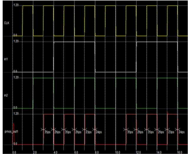
Fig.5. Output Waveform for DTV Technique
