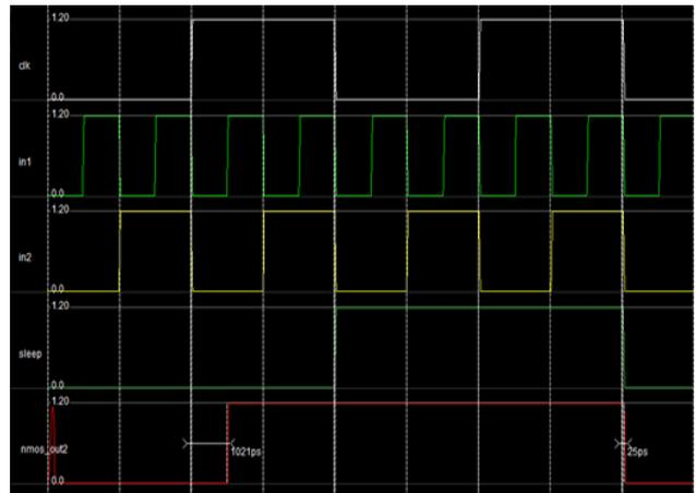
Fig.7. Output Waveform for Sleep Switch Based Domino Circuit
