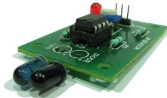
Fig 7.5: IR Proximity Sensor
