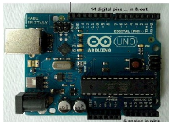
Fig 7.1: Arduino Uno Board
