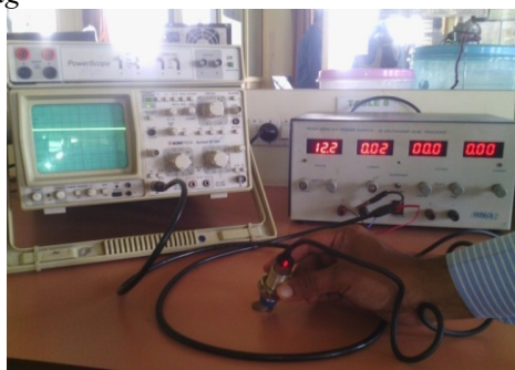
Fig 8. Testing of Inductive Proximity Sensor
