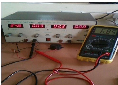
Fig.10. Testing of signal conditioning circuit for Buzzer
