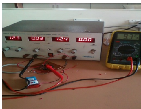
Fig 9. Testing of signal conditioning circuit for temperature sensor
