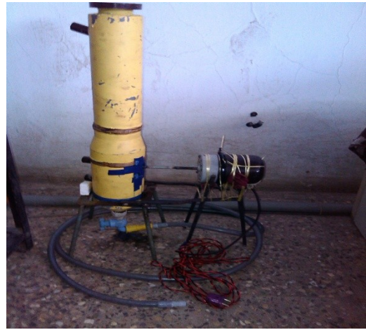
Image 2 :- The filtration cum aeration unit as used in the experiment
