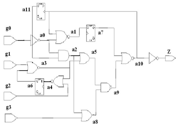
Fig 1. S27 A example circuit for testing
