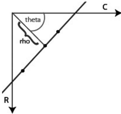
Fig.1. The algorithm of Hough Transform.
