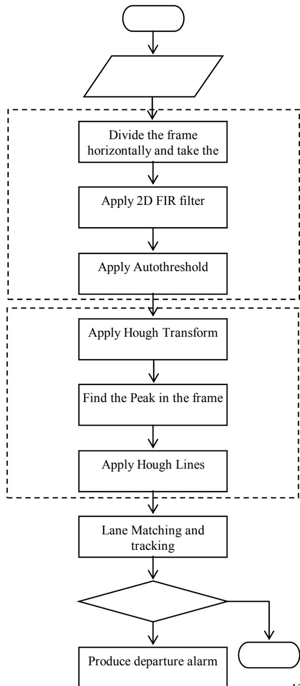
Fig.2. System block diagram of the proposed system.
