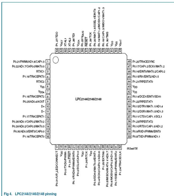
Figure 4. Pin Configuration LPC2141/42/44/46/48
