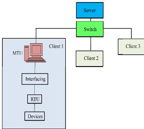
Figure 1: Block diagram of SCADA system
