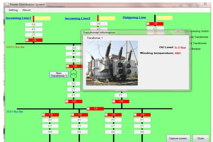
Figure 5: Showing the status of main transformer 1
