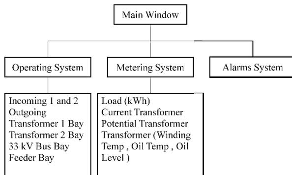
Figure 3: Flow diagram of monitoring system
