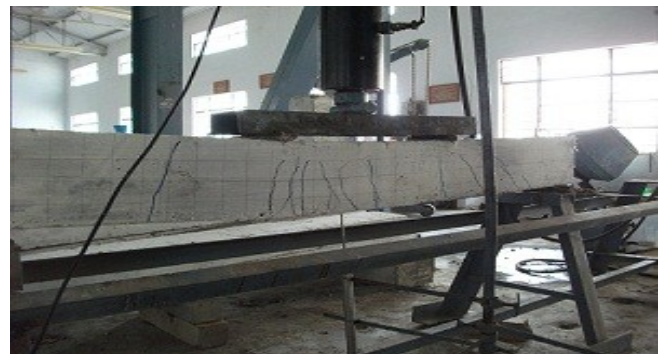
Fig 3 Beam Test Setup under Two point loading
