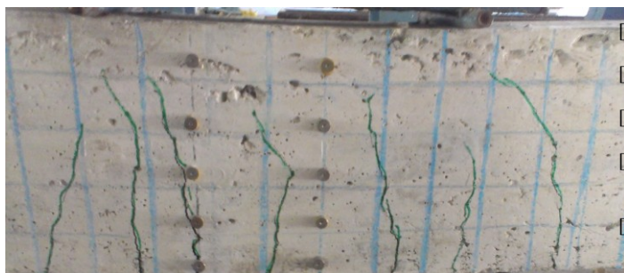
Fig 5(c) Failure pattern for BS0.75P0.25
