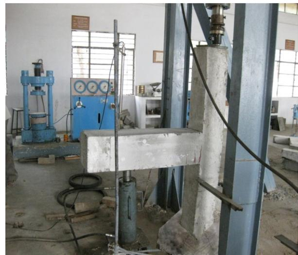
Figure 3 Experimental set up for beam column joint
