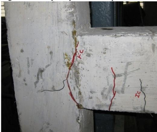
Figure 5(a) Failure in BCP0.5
