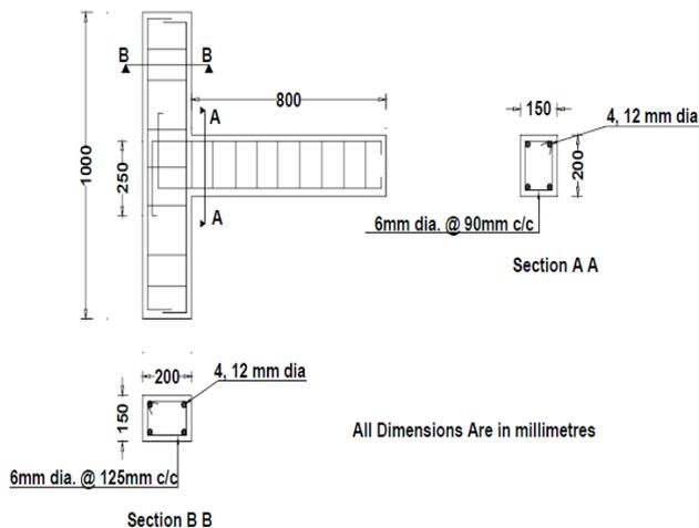
Figure 1 Reinforcement detailing for exterior beam column joint
