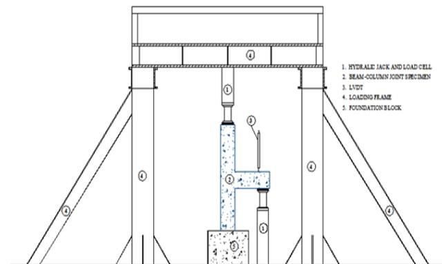
Figure 2 Schematic Diagram of Cyclic loading Test Set-up
