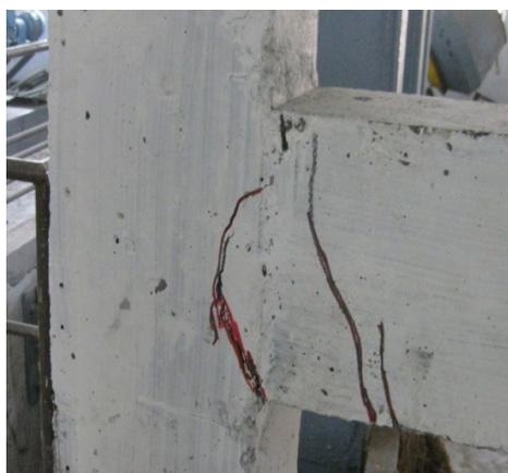
Figure 5(c) Failure in BCS0.5P0.5
