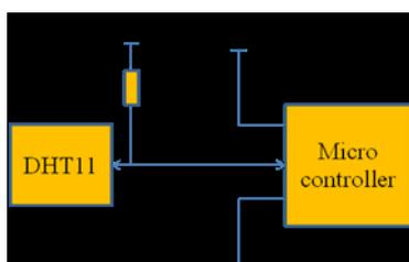
Fig. 2.Connection between MCU and DHT
