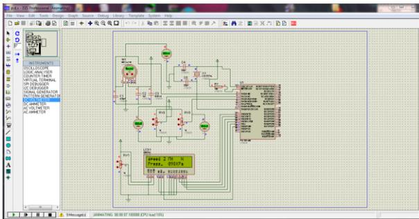
Fig. 6. Screenshot for the simulation result of pressure (100Kpa), wind speed (2MH) and direction (NORTH)
