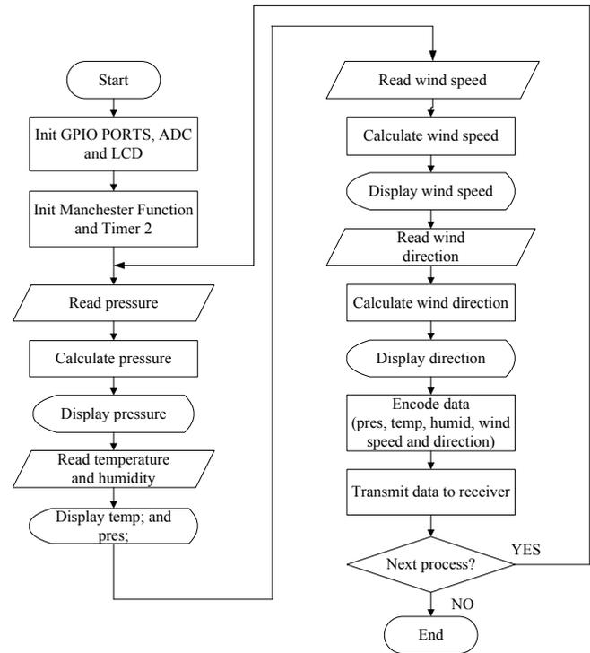
Fig. 4. Flowchart for sensing unit in transmitter wireless weather station
