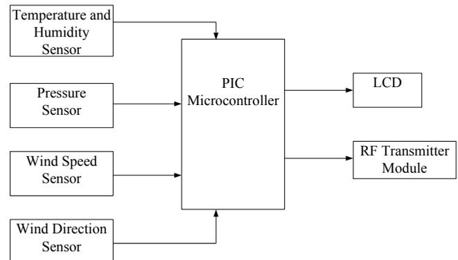
Fig. 1. Block Diagram of Sensing unit in Transmitter for Wireless Weather Station
