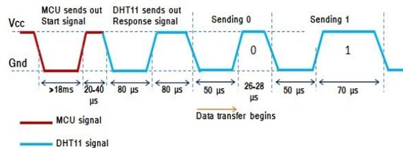
Fig. 3. Communication Process of MCU and DHT11
