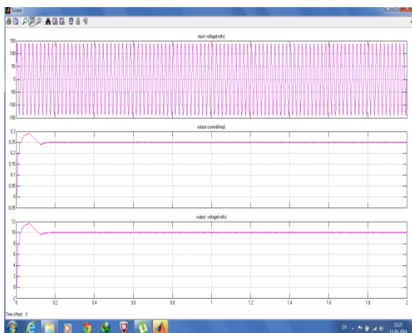
Figure 6. Output Voltage and current with 140 V input voltage at load resistance 40Ω
