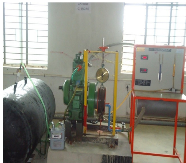
Fig.1 Experimental setup of biogas-fueled C.I engine
