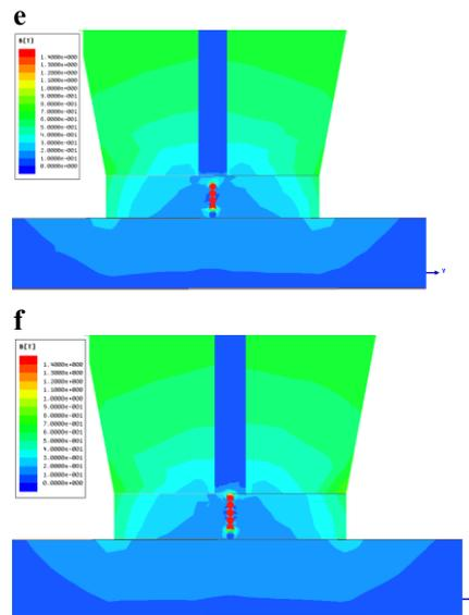
Fig.5 Shows the magnetic flux density on a copper workpiece (a) without any CIP, (b), (c), (d), (e), (f) with 1,2,3,4,5 CIPs added respectively.
