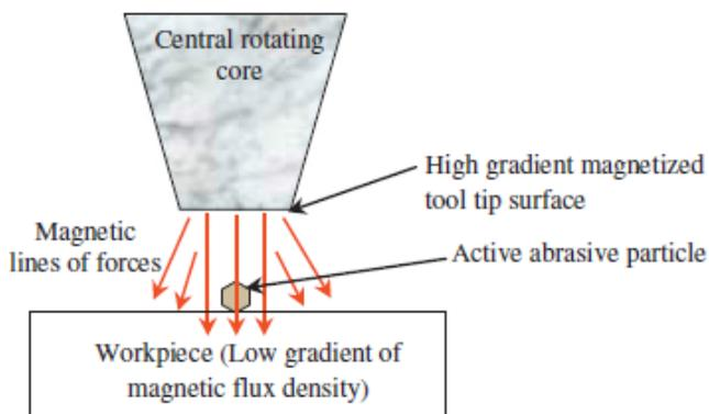
Fig.2 Interaction of abrasive particle with workpiece surface due to repulsion by a high gradient magnetic field.
