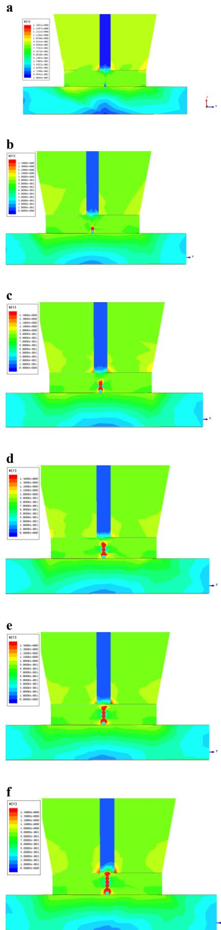
Fig.4 (a) shows the magnetic flux density for a ferromagnetic workpiece with (a) no CIP, (b), (c), (d), (e), (f) with 1,2,3,4,5 CIPs.
