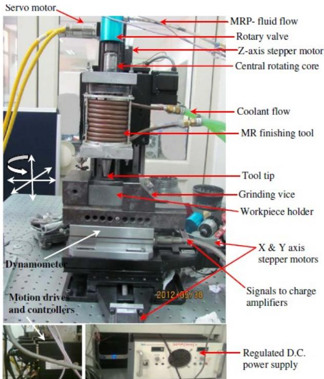
Fig.1.BEMRF set up.
