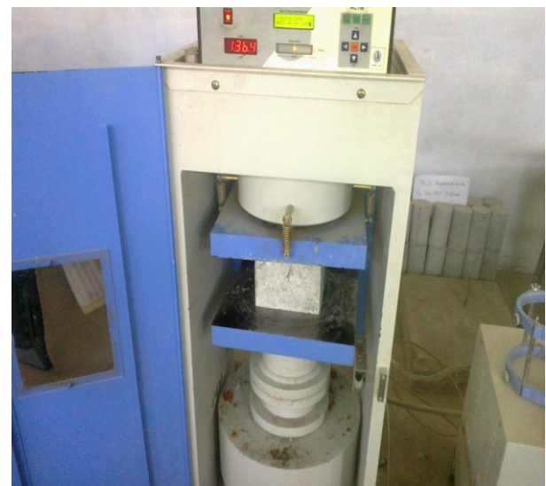
Figure 3.4 Compressive strength test in progress
