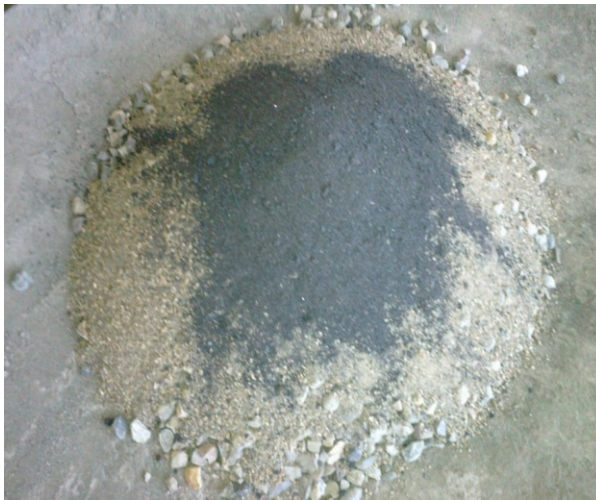
Figure 3.1 Dry mix of cement, sand, aggregate and iron slag
