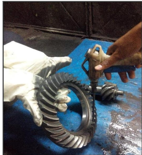
Figure 1: Trial test of compressed air on Lapped Job
