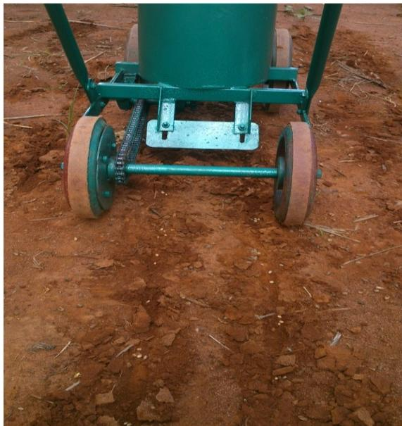
This equipment consists of cylindrical shape container in which the seeds can fill. The capacity of this container is up to 10kgs to 12kgs. The container is attached on the four wheeled carrier assembly. The
