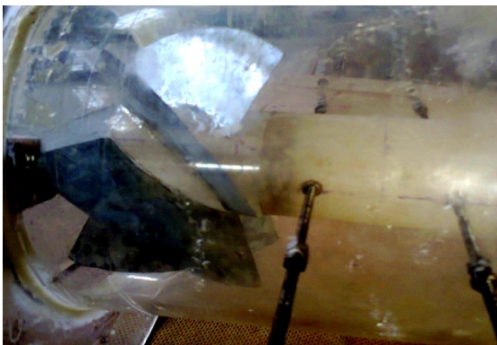
Fig.2 Eight Rotating vane Swirler
