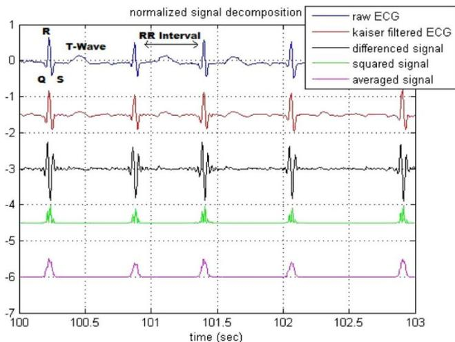
ECG main points and signal processing for QRS detection
