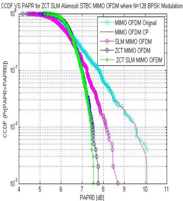
Fig. 10 CCDF Vs PAPR of ZCT-SLM based Alamouti STBC MIMO-OFDM system with ZCT MIMO-OFDM system, SLM MIMO OFDM system and conventional MIMO-OFDM system with and without adding cyclic prefix
