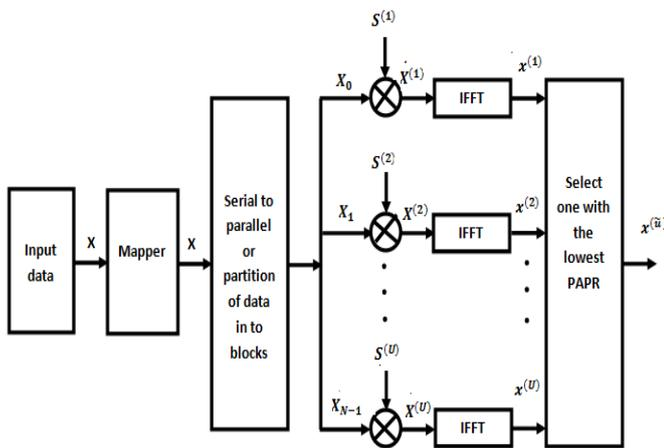
Fig. 3. Block diagram of SLM based OFDM system.
