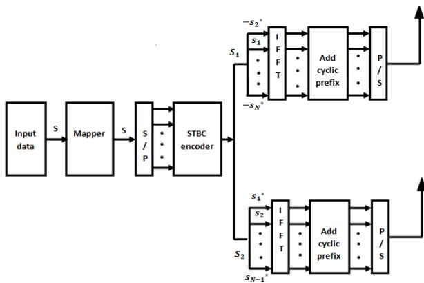
Fig. 5. Block diagram of Alamouti STBC MIMO- OFDM system.
