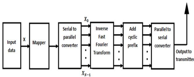
Fig. 1. Block diagram of Conventional OFDM system
