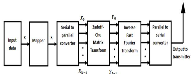
Fig. 2. Block diagram of ZCT based OFDM system
