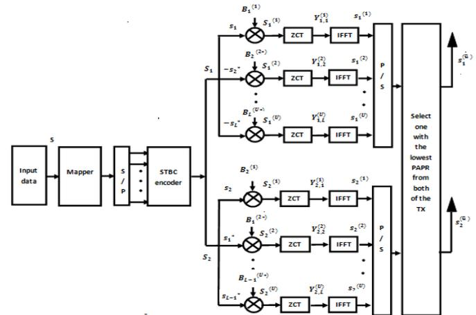
Fig.8. Block diagram of ZCT-SLM based Alamouti STBC MIMO-OFDM system
