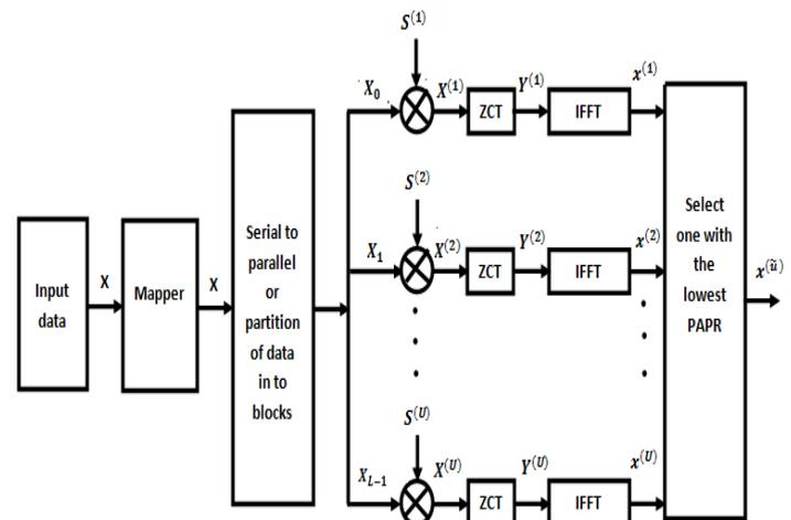
Fig. 4. Block diagram of ZCT-SLM based OFDM system.
