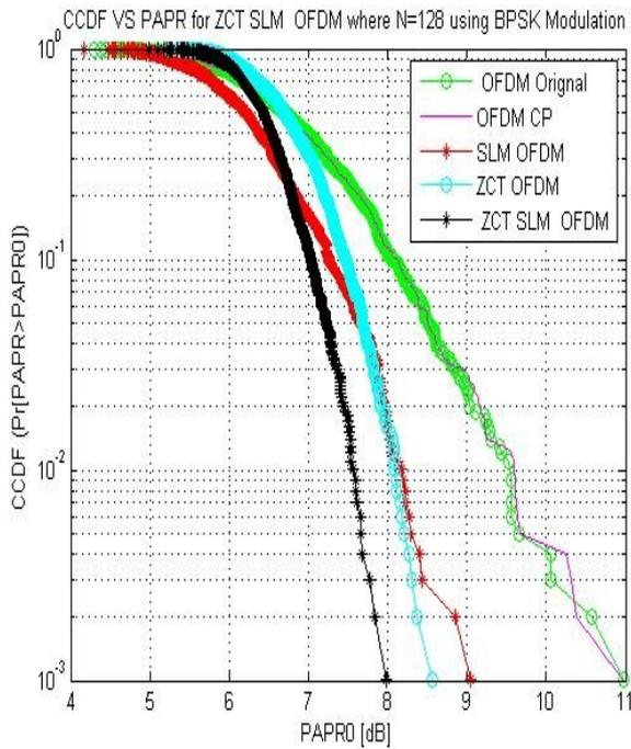
Fig. 9 CCDF Vs PAPR of ZCT-SLM based OFDM system with ZCT-OFDM system, SLM-OFDM system and conventional OFDM system with and without adding cyclic prefix
