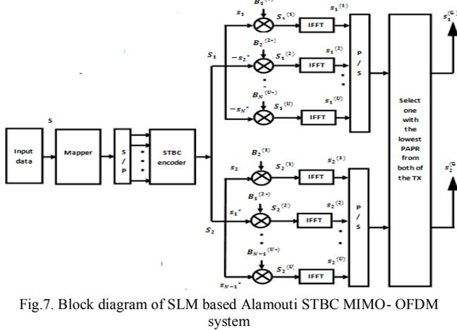
Fig.7. Block diagram of SLM based Alamouti STBC MIMO-OFDM system
