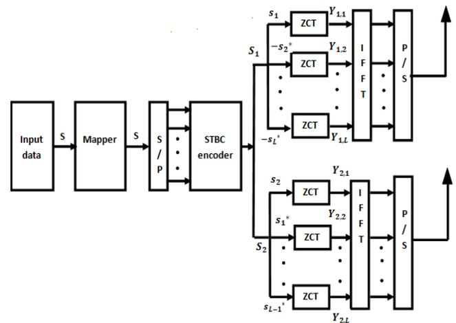
Fig.6. Block diagram of ZCT based Alamouti STBC MIMO- OFDM system
