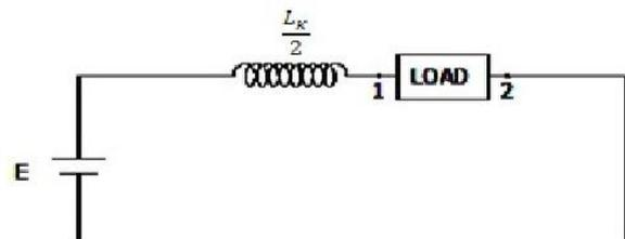
Fig. 8: Thevenin equivalent circuit of case-2
