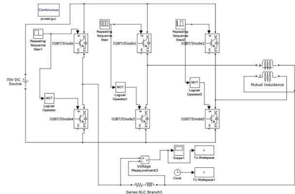
Fig. 13: Simulation of five level inverter with coupled inductor for R-L load
