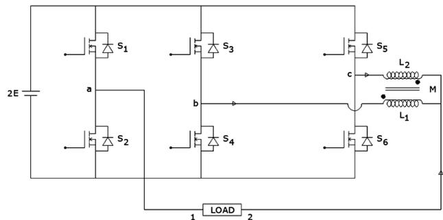
Fig. 1: Single-phase five-level inverter
