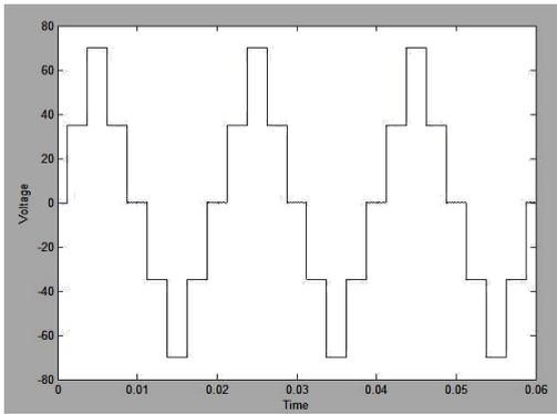
Fig. 14: Simulation result of five level inverter with coupled inductor for R-L load
