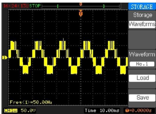
Fig. 15: 70V Five level AC output voltage
