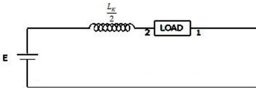
Fig. 10: Thevenin equivalent circuit of case-3
