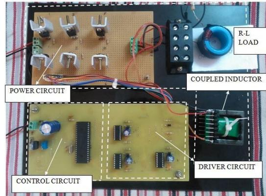
Fig. 16: Laboratory prototype of the single phase five level inverter
