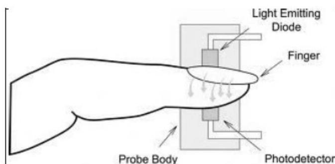
Fig 3: Transmission PPG Sensor
