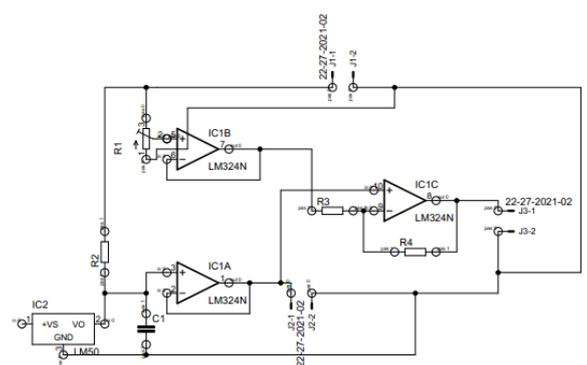
Fig. 7: Temperature Sensor Module
