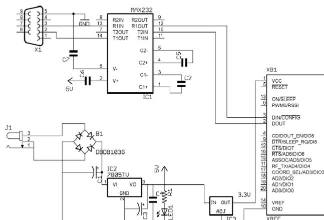
Fig 8 : Radio Transreceiver
