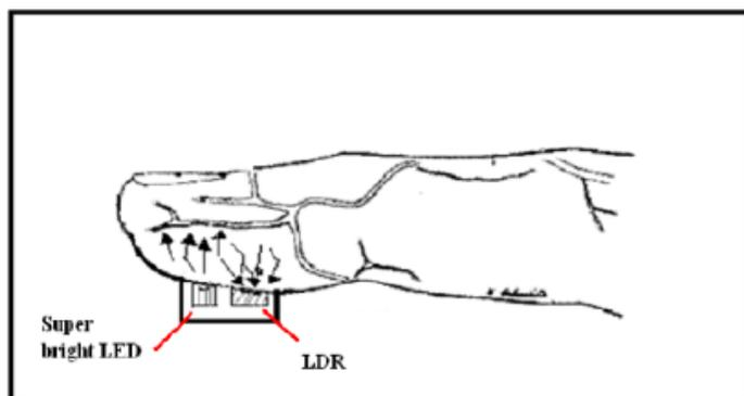
Fig 2: Reflectance PPG Sensor.
