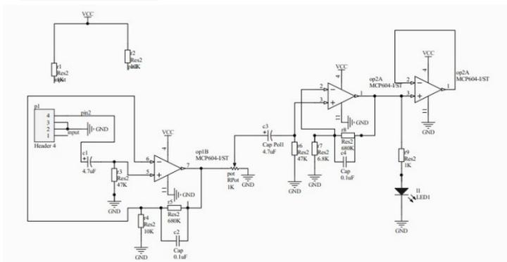
Fig. 6: Pulse Sensor Module
