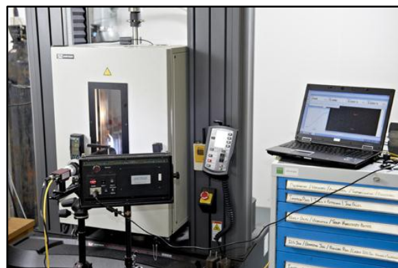
Fig. 1 Video gauging test set-up
