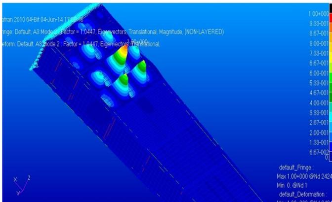
Fig: 4 Buckled shape of critical panel
