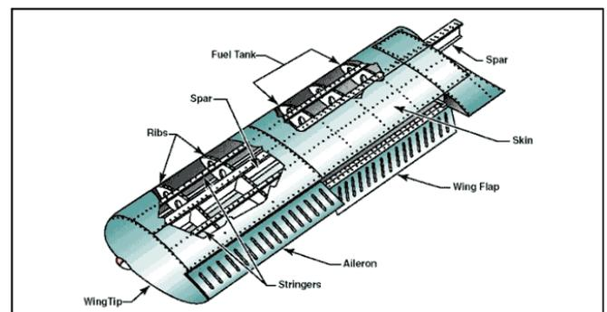
Fig: 1 Parts of a wing
