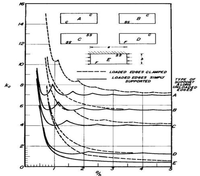
Fig: 5  $k_c$  values for different edge support conditions
