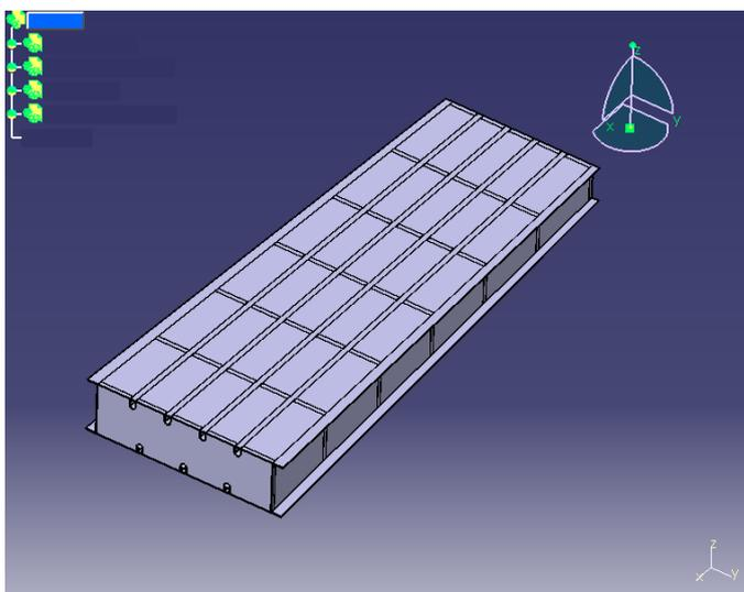
Fig: 2 CAD model of the wing box
