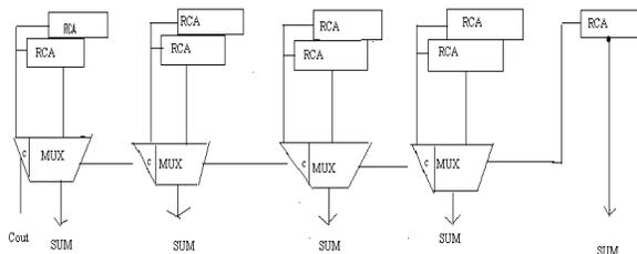
Fig (B) : CSA with Proposed RCA Circuit
