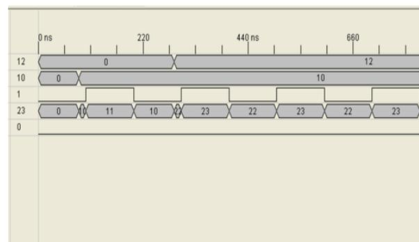
This is the screen shot of CSLA with BEC simulation results. Here inputs are A,B and Ci, outputs are SUM and Cout.
