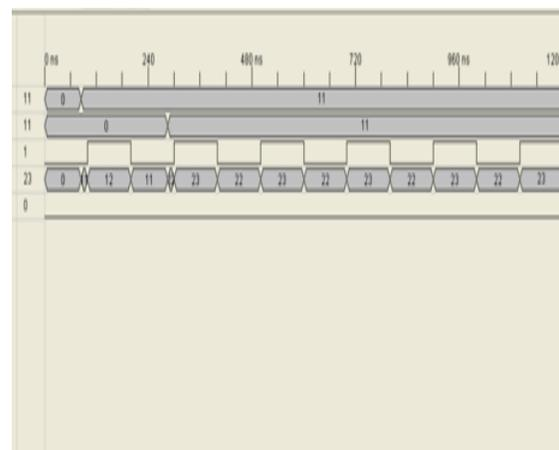
The Fig.(C) shows the simulation results of 16 bit CSA with RCA,these values are calculated by Xilinx software. Whereas A,B and Cin are input values, these values generate the corresponding SUM and Cout values.
