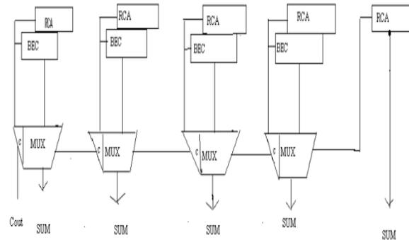
Fig (B): Basic building block of CSLA with BEC
