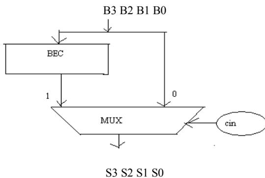
Fig (A) : BEC with MUX
