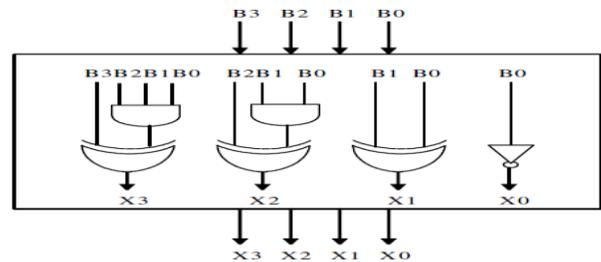
Fig.1.1.Binary to Excess Converter
