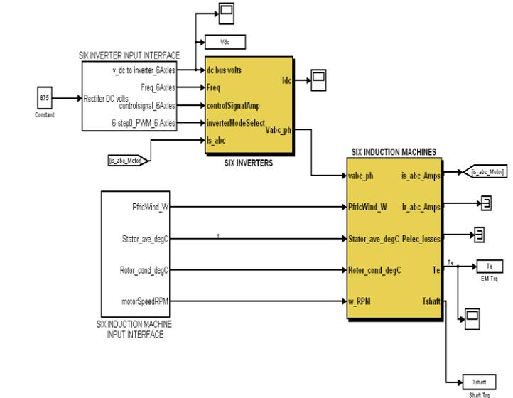
Figure 3 : Snapshot of the SIMULINK model – 6 inverters and 6 machines using vectorized modeling approach.
