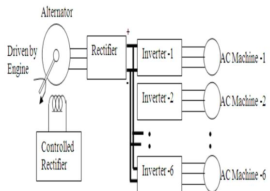
Figure 1: Schematic of an AC propulsion System
