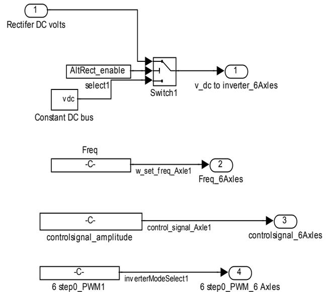
Figure 4: Internal details of the six inverter input interface block
